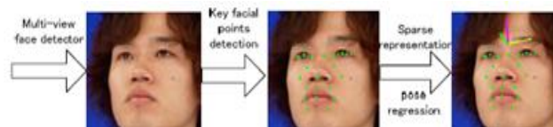
Figure 9. Flowchart of the pose estimation system
